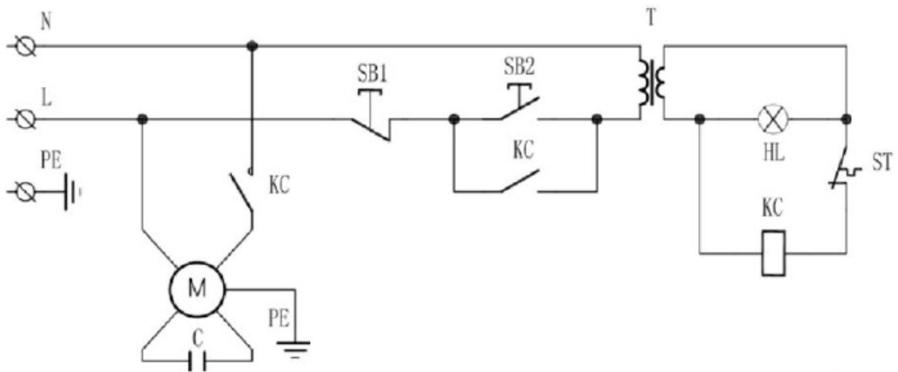
M - Motor, C - Capacitor, T - Transformador, SB - Interruptor principal
