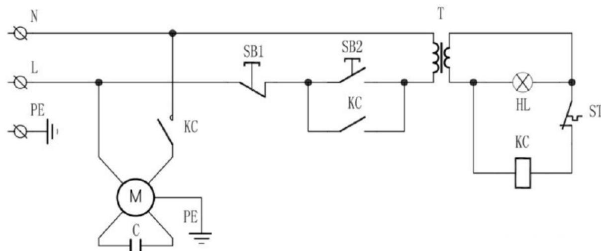
M - Motor, C - Capacitor, T - Transformador, SB - Interruptor principal
